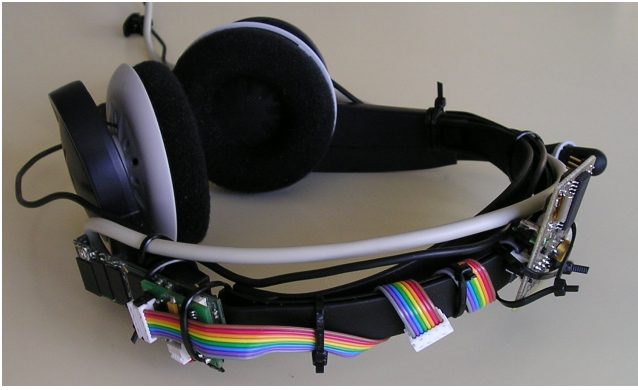
Figure 1: Sound spatializer prototype, with Gumstix (bottom left) and compass (right) attached to headphone.
