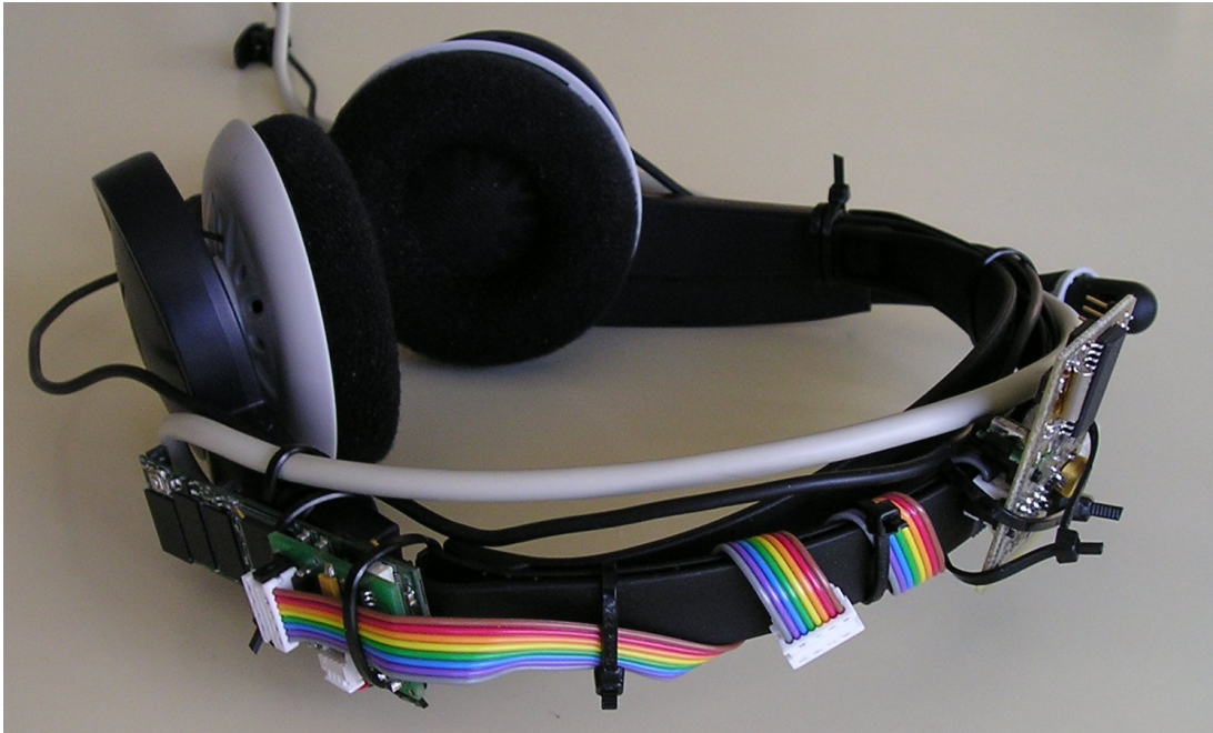
Figure 7.1: Sound spatializer prototype, with Gumstix (bottom left) and compass (right) attached to headphone.
